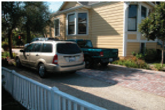
Examples of parking surfaces with porous pavement
