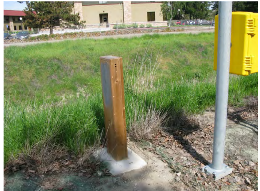
Example of an automated bicycle/pedestrian counter installed next to Alamo Canal Trail north of the I-580 undercrossing.
