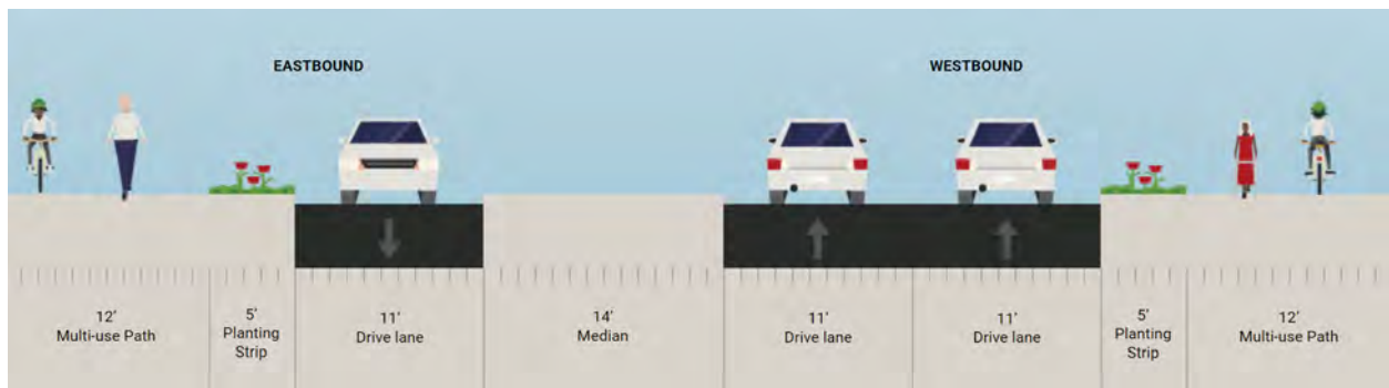
Plate 6 Option E – Westbound and Eastbound Class I Multi-Use Path with Narrowed Median
