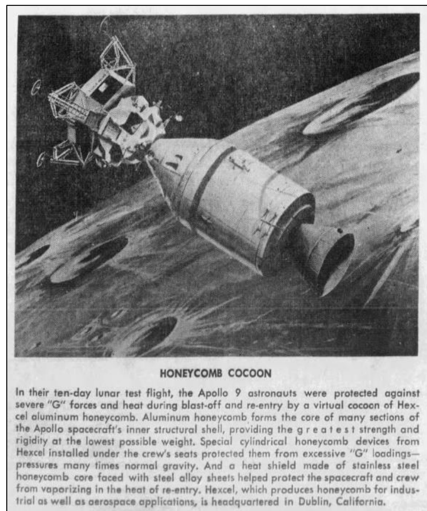
Plate 7: Drawing and description of Hexcel honeycomb for Apollo 9 (Source: Contra Costa Times 1969 March 28).
